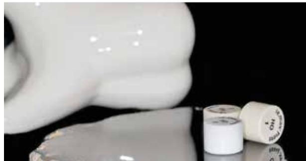
**Fig 20** e.max HO ingots.
